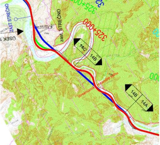
The figure shows the proposed route of the modernized line. The red route follows the current route, the blue represents the solution with the highest line speed and the greatest distance reduction.
