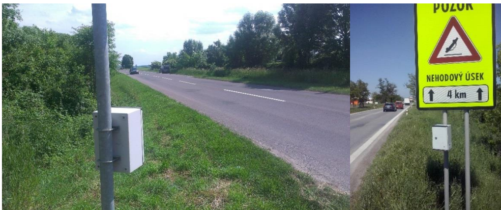
Figure 7 Example of placing automatic traffic counter for the traffic count
