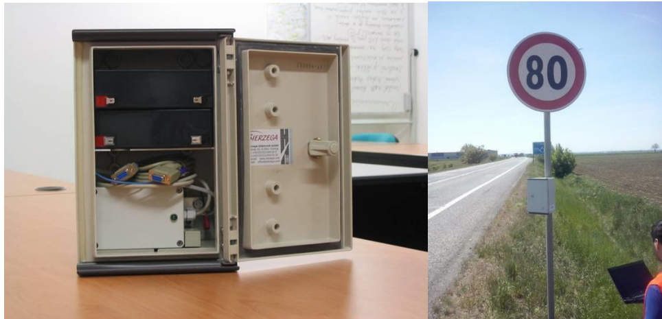
Figure 21 Automatic traffic counter Sierzega SR4 and installation example
