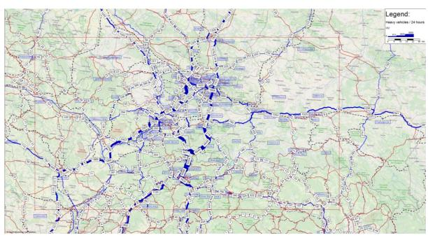
Figure 1 Road network load by freight traffic in the TRITIA model, zero scenario /2030/
