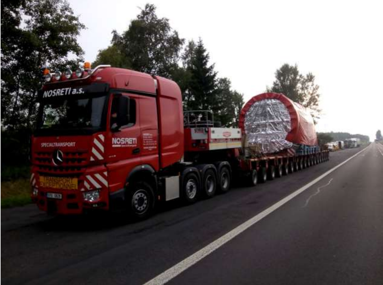
Figure 24 – Transport of stator from Pilsen to Mochovce
