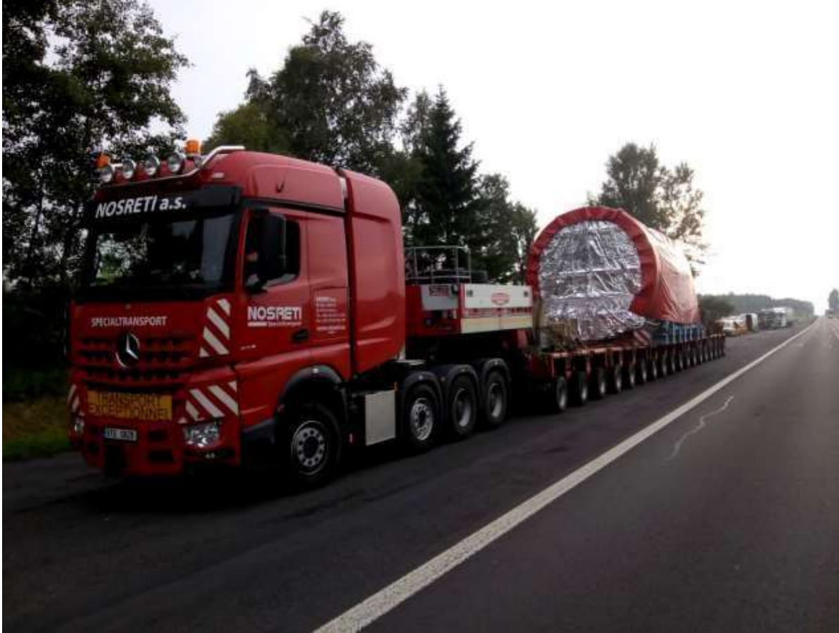
Figure 24 – Transport of stator from Pilsen to Mochovce
