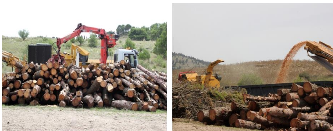
Figure 9 – The chippers in action in two different phases of work (logs loading and chipping) in dedicated squares out of forest in Sicily.
