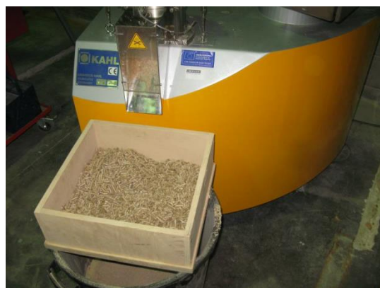
Figure 4. Sample of experimental pellets manufactured with KAHL press with plane matrix of 50 kg/h capacity. Own source.
