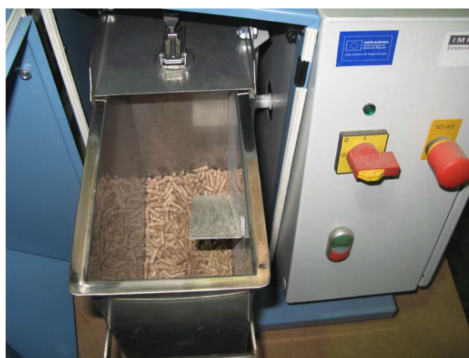
Figure 5. Test of mechanical durability with Bioenergy TUMBLER Series following EN 15210-1. Own source.
