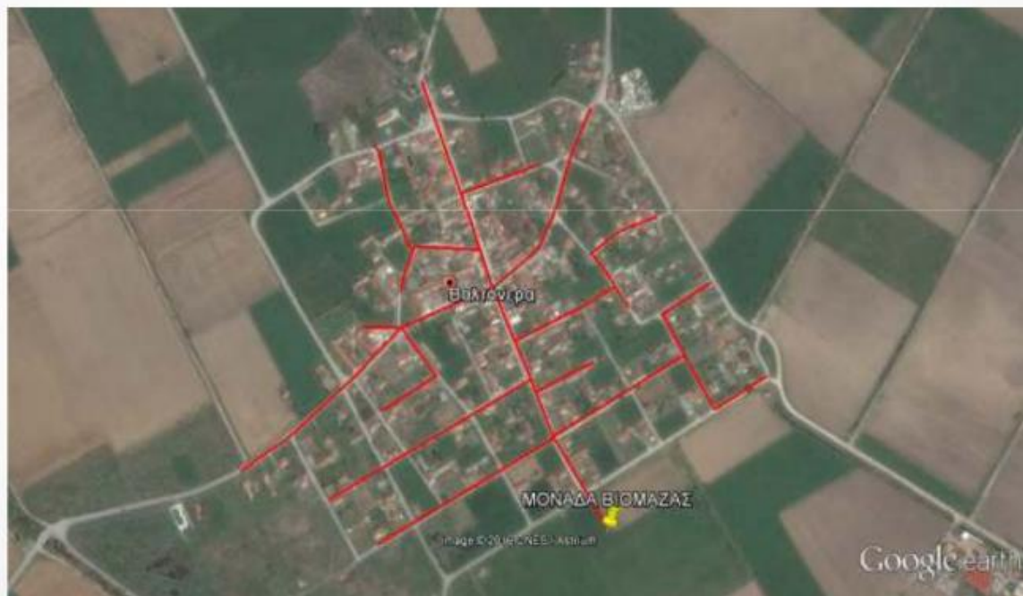
Image 6.7 The design of the biomass district heating system of a village in Amyntaio area.
