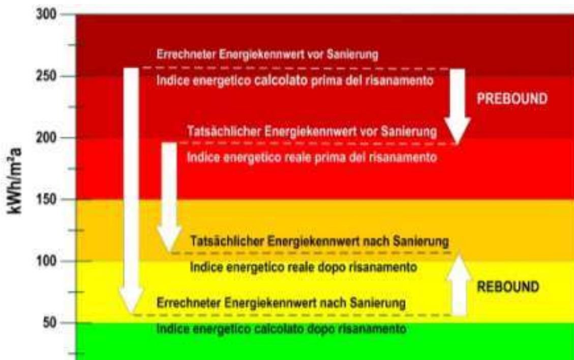
Figure 4.1.b: Prebound and rebound. Study carried out by CasaClima / KlimaHaus Agency. The image shows the real energy ratio before of the intervention (prebound) and after the intervention (rebound).
