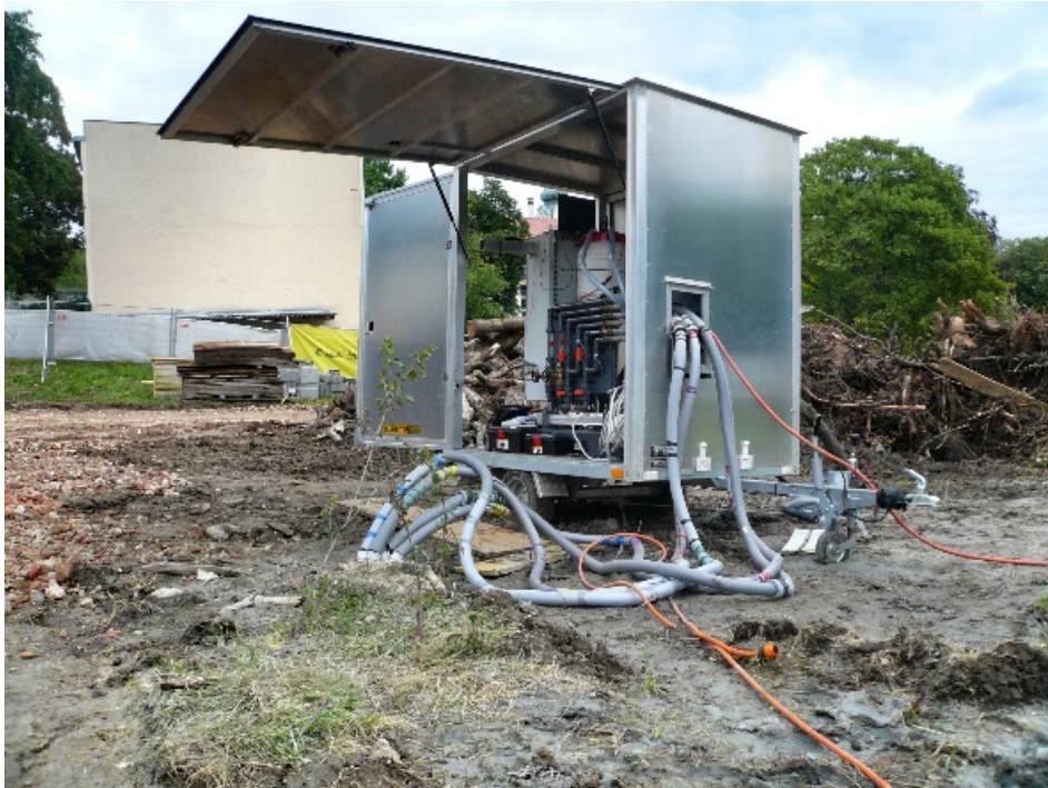
Figure 5: TRT Device #1 (LP - Geologische Bundesanstalt).
