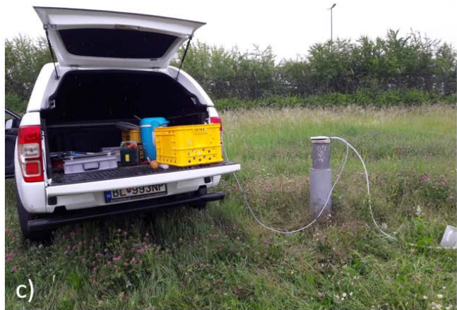
Figure 7. Groundwater sampling. a) Documentation of on-site measurements. b) Sampling equipment - Surface water sampler. c) Sampling equipment - Submersible pump inside well.
