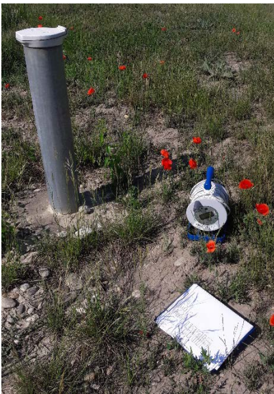
Figure 1. Equipment for manual groundwater temperature and water level measurements (well dipper and notepad) next to an observation well.
