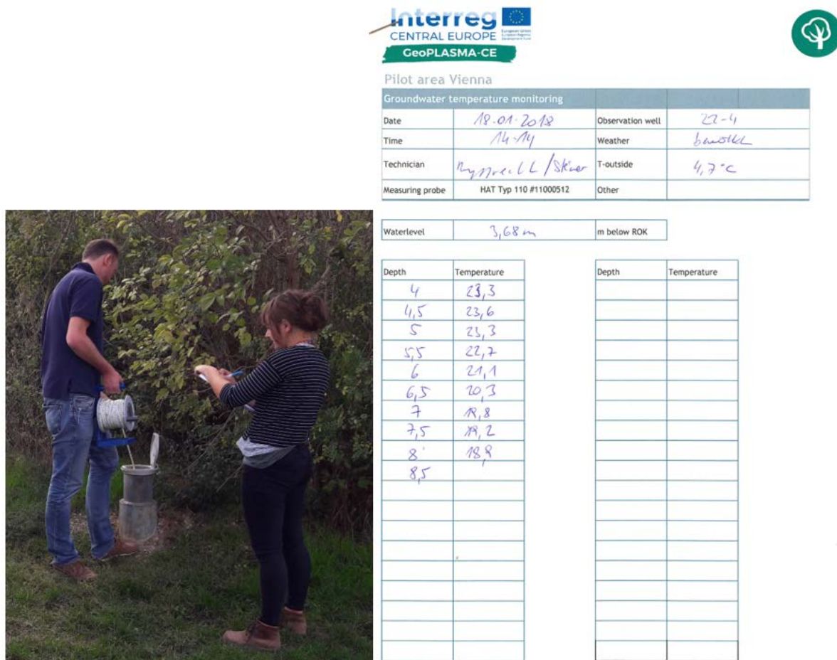
Figure 4. Procedure of taking manual groundwater temperature measurements in 50 cm depth intervals and documentation sheet.
