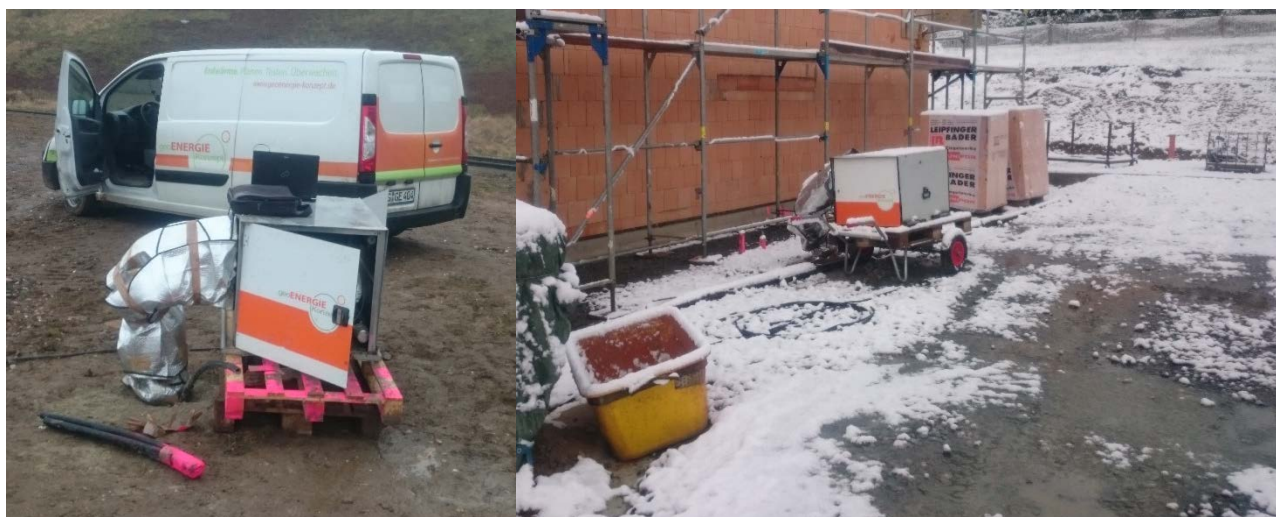
Figure 2: Thermal Response Test device
