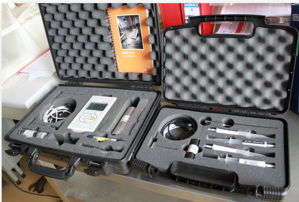
Fig. 10. PGI-NRI KD2 Pro thermal conductivity analyzer.
