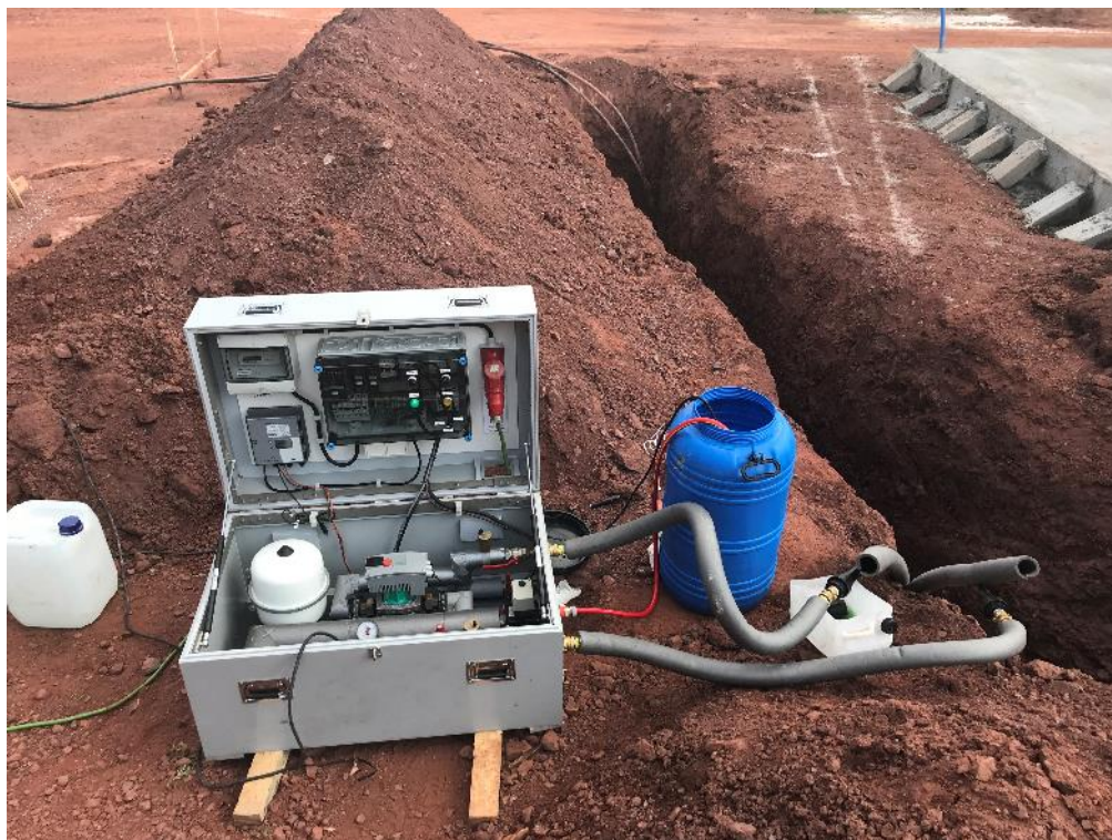
Fig. 13. PGI-NRI TRT probe (Model GeRT produced by UBEG).
