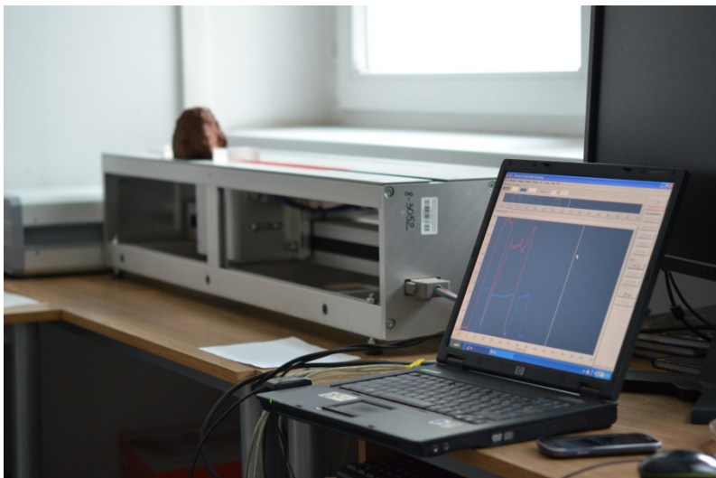
Fig.4. Thermal Conductivity Scanner (TCS) in PGI-NRI geophysics laboratory in Warsaw.
