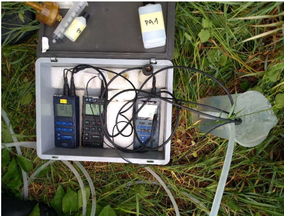
Figure 7: Setup of the WTW multimeter tools with four different sensors for groundwater on-site analysis.
