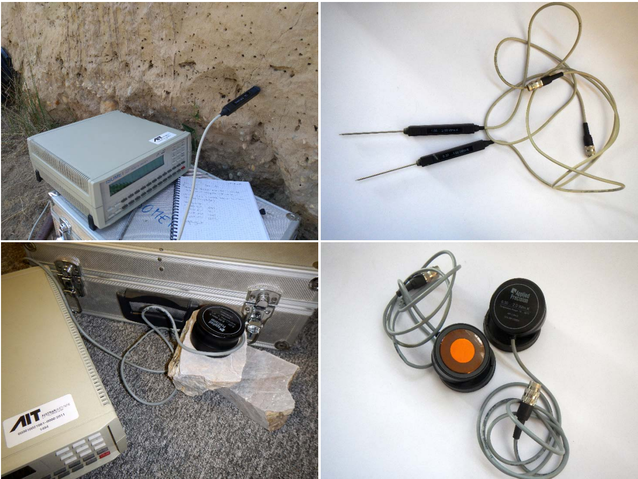
Figure 9: Measurement devices for the determination of thermophysical properties in the PA Bratislava. On top: Left: The Isomet 2104 during measurement. Right: Needle probes used for the investigation of soft rocks. Bottom: Left: The Isomet 2104 during a measurement in the laboratory for hard rock investigations. Right: Surface probes for the investigation of hard rocks.
