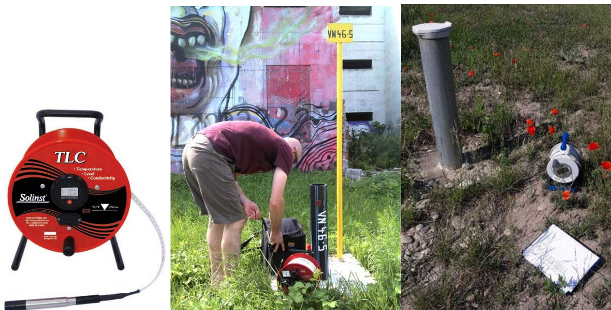
Figure 2: Left and middle: Solinst groundwater table depth meter with temperature and EC measurement probe used for manual measurements in the Slovak part of the pilot area. Right: Equipment for manual groundwater temperature and water level measurements in the Austrian part of the pilot area.
