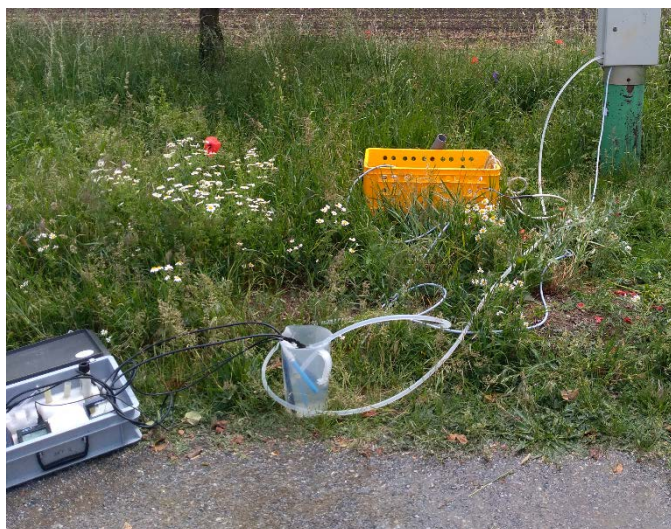
Figure 6: Measurement with the WTW logger in beaker.
