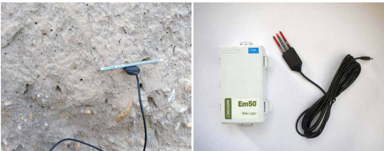
Figure 10: Measurement device for the determination of soil moisture and temperature in the PA Bratislava. Left: Measurement arrangement of the sensor in the field. Right: The Em50 data logger and used soil moisture and temperature sensor (5TM).
