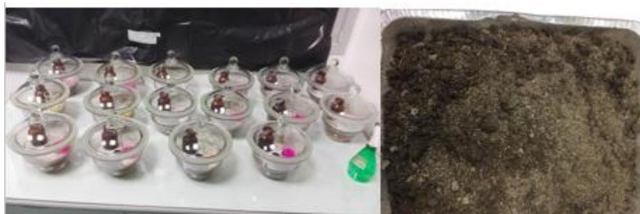
**Figure 12. A.** Sealed glass containers to measure the gas emission during the biodegradation of plastic in soil
