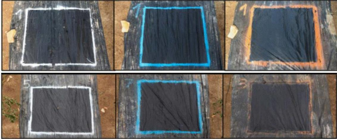
**Figure 13. Top row:** Control areas in the first row of each type of mulch. From left to right: Ecovio (white), Biomulch (blue), LDPE (orange). **Bottom row:** Mulch status 192 days after placement. (Image source: IFAPA, Instituto de Formacion y Investigacion Agraria y Pesquera – Junta de Andalucia, Interreg Med Reinwaste Project pilot activities.)
