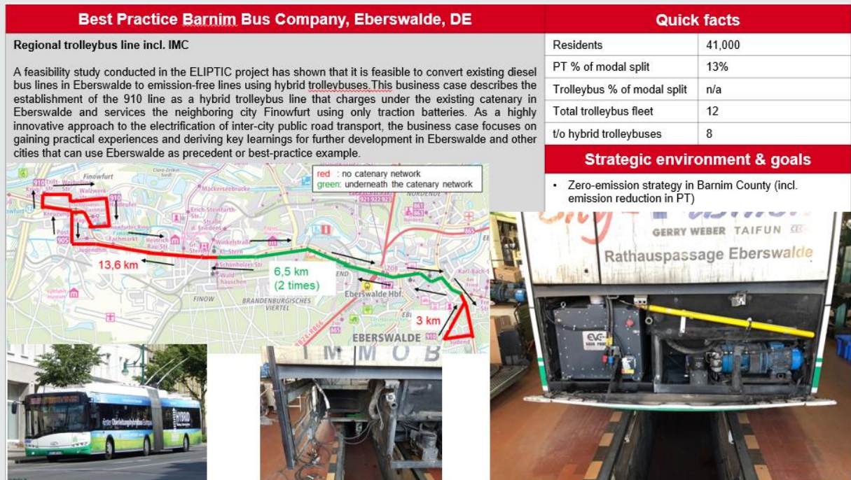
Figure 14: Best-Practice BBG, Eberswalde for IMC realisation to replace existing diesel bus line with trolleybus operation - based on retrofitted battery-trolleybuses line (source, trolley:motion, 2020)
