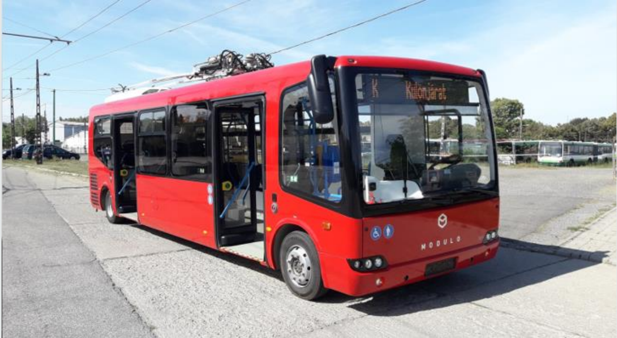
Figure 15: Modulo EP095T, composite framed midi-bus with IMC (source: SZKT 2020)
