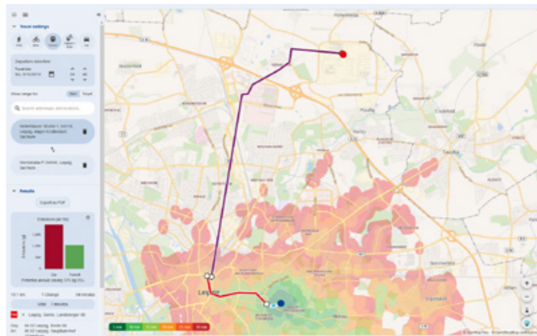
Above: Screenshot of the REACHIE integrated mobility platform showing various modes of travel for a selected route and the associated CO 2 savings in a bar graph on the left margin (2019, MDV).
