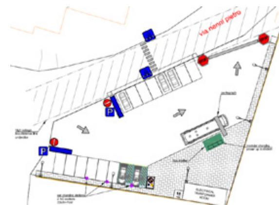
Figure 15: New mobility hubs: layout of the terminal at Largo Nenni, Parma (Source: TEP 2020)
