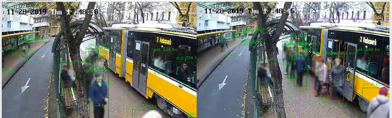
Pictures from Szeged showing camera-based validation of the WiFi passenger counting method. Source: SZKT.
