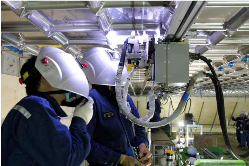
Mini welding robots can operate in areas inaccessible to humans. A magnetized body allows them to suspend from panels and ceilings.
