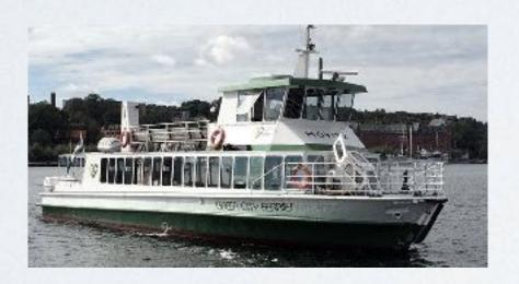
E/S Movitz, the world's first supercharged passenger ferry operates for an hour and recharges in 10 minutes.
