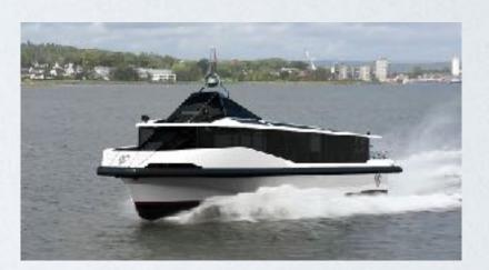
BB Green 24, An electric or hydrogen FSV vessel for 147 passengers plus 26 bikes, service speed of 30 knots with ultra-low wakes of 26cm
