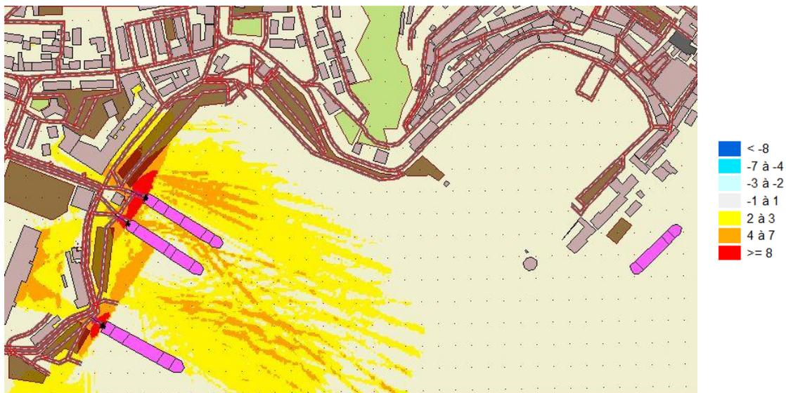
FIGURE II.3: PORTOFERRAIO –CARTE DE L'EMERGENCE (DIFFERENCE ENTRE LE BRUIT TOTALE MOINS CELUI CAUSE PAR LE TRAFIC ROUTIER)
