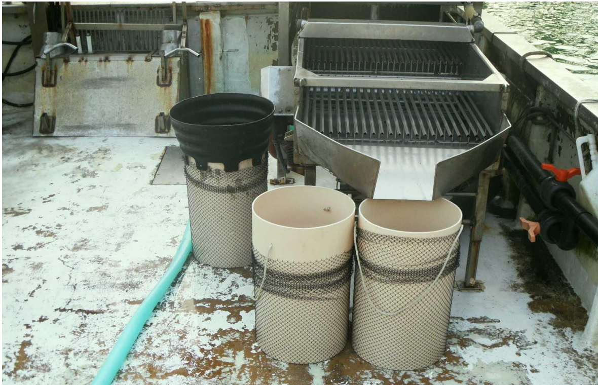
FIGURE 5-4. The bins for the net cuttings installed onboard the maricultural vessels (Photos © Walter De Walderstein).
