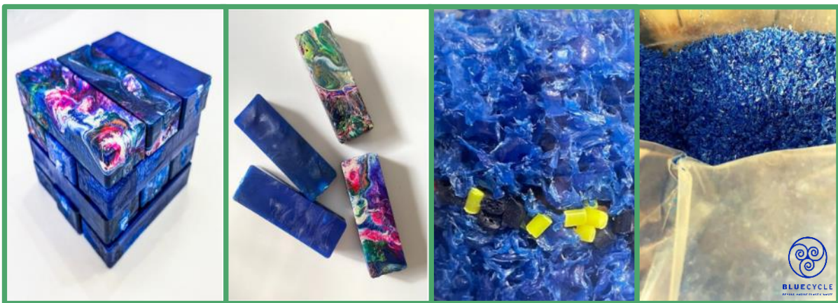
FIGURE 4-5. The end product from the mechanical recycling of mussel nets (Photos © iSea).
