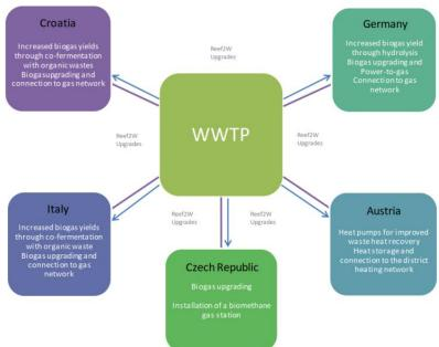
Focus: Co-digestion with biowaste, biogas upgrading, heat capture, power-to-gas
