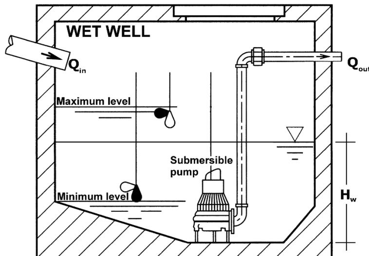
Figure 1. Classic wet well with submersible pump.
