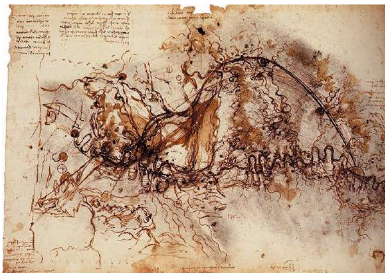
Fig. 1. Leonardo’s deviation of the Arno River; bypassing a stretch of the river with an artificial canal (never put into practice). (Source: Royal Collection Trust at https://www.royalcollection.org.uk/collection/912279/a-scheme-for-a-canal-to-bypass-the-arno ).
