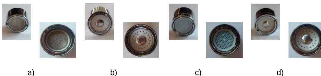
Fig. 1. Characteristics of the different aerators: a Aerator A (aerated flow; Q = 4.7 l/min); b Aerator B (spray flow; Q = 3.9 l/min); c Aerator C (aerated flow; Q = 3.4 l/min); d Aerator D (spray flow; Q = 2.0 l/min).
