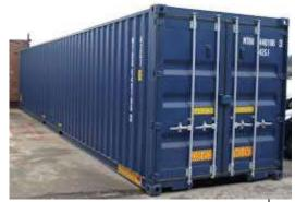
Furthermore, containers can be Dry Van (DV/DB), High Cube (HQ/HC), Flat Rack (FR), Refrigerated-reefer (RF), and Open Top (OT), and these models in various configurations.
