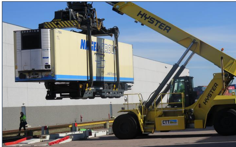
19. Figure Loading a non-cranable semi-trailer with the NIKRASA system SOURCE: HTTP://WWW.NIKRASA.EU/DE/STARTSEITE.HTML
