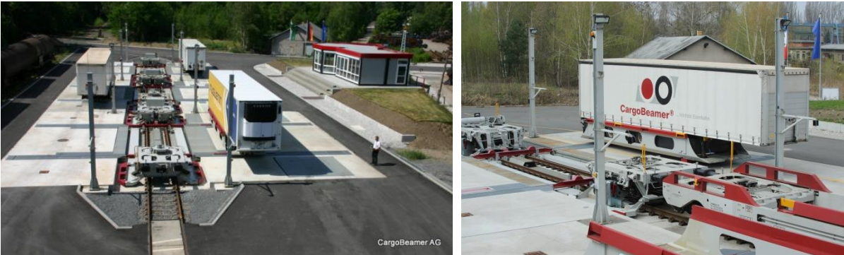
21. Figure Loading/unloading with the CargoBeamer system SOURCE: HTTP://WWW.CARGOBEAMER.FR
