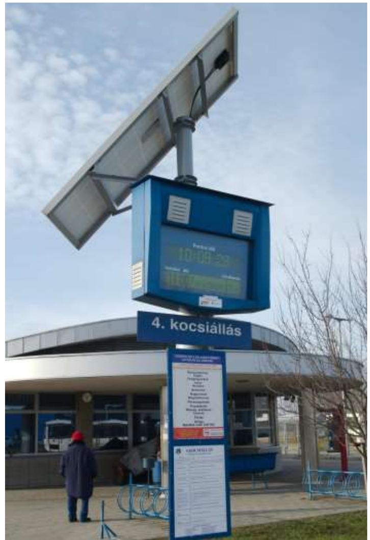
Figure 6: solar panel display at the bus station (source: KTI)
