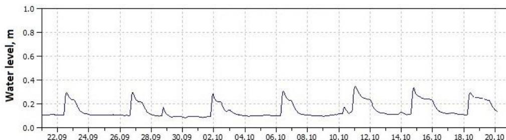
**Figure xx. The example of hydropeaking in Tenenys river below Ramučiai HPP dam for period September 21 to October 20, 2020. Every few days the minimal sanitary water level is flushed by the accumulated water suddenly raising water to +20 cm. Data are taken from Lithuanian Hydrometeorological Service automatic water station in Tenenys River at Miestaliai village <http://www.meteo.lt/lt/hidroinformacija>**
