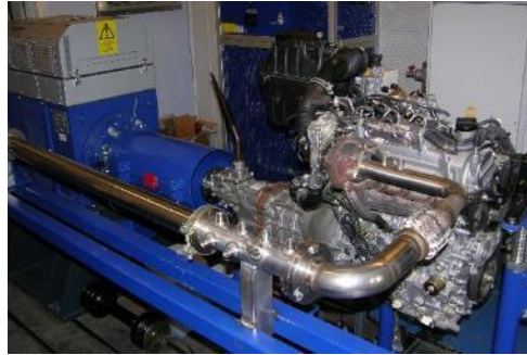
3 fully equipped engine benches for emissions testing
