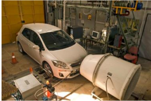
Chassis dyno for vehicle emissions testing
