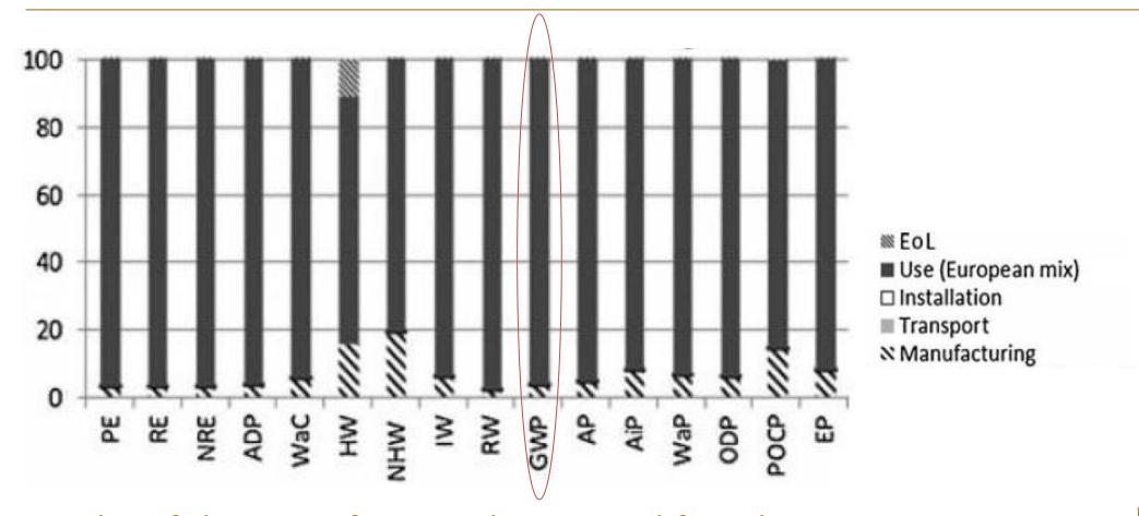
Results of the LCA of an LED luminaire lifecycle in EU (Tähkämö et al. 2013)
