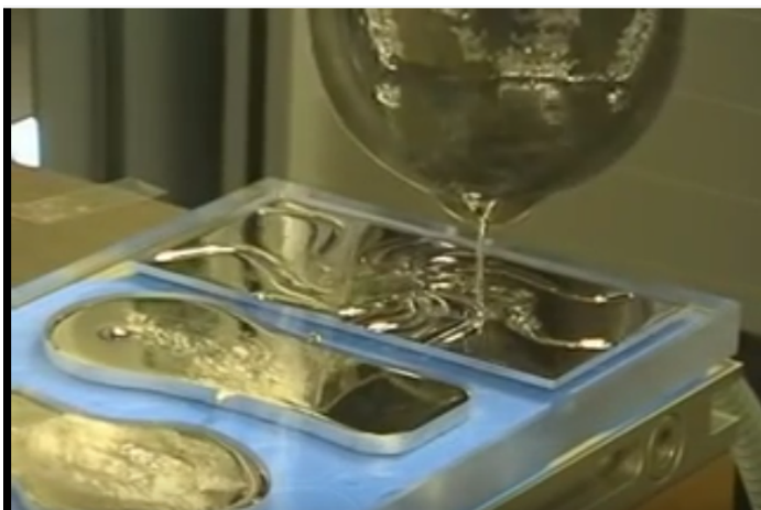
Figure 21: Weiguss liquid metal as clamping alloy
