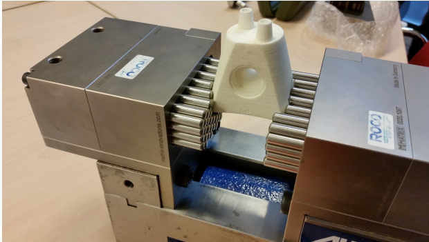
Figure 31: matrix clamp with (polymer) user case Hittech
