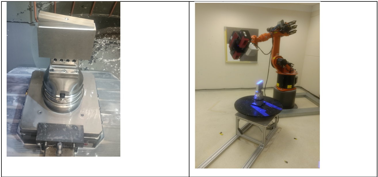
Figure 1 left; the Fast Prototype object during fabrication by using a 5 axis CNC milling machine at Hitech Bihca. Right: The object during 3D scanning by using a robotized measuring cell at Argon measuring solutions
