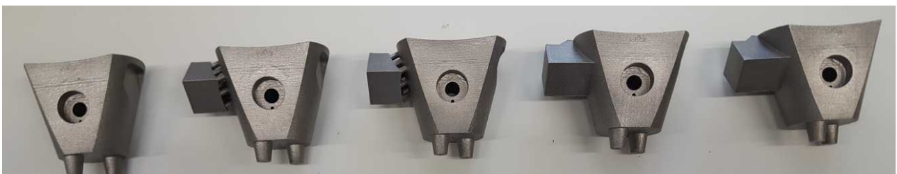
Figure 8: Left: mirror object without handle; middle:, Mirror object with handle and struts interface; right: mirror object with solid handle.
