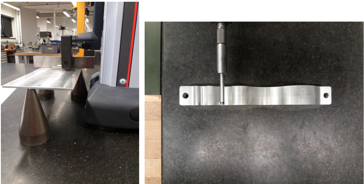
Figure 41: Left: measurement of thickness of sample with height measuring instrument. Right: measurement of roughness with the Perthometer C5D.
