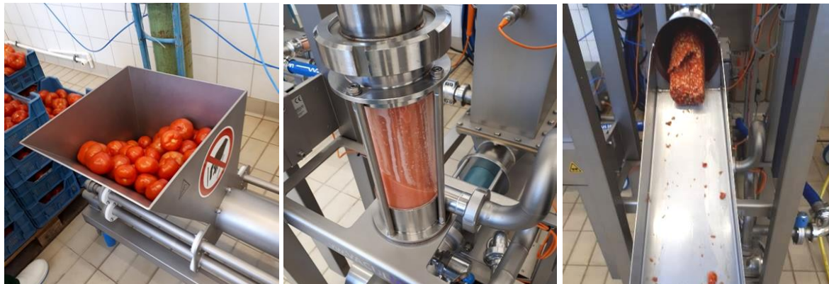
Figure 2: Starting material in the Multicut before cutting & milling (left), juice extraction in the VacullIQ (middle) and tomato press cake coming out of the VacullIQ as solid fraction (right)
