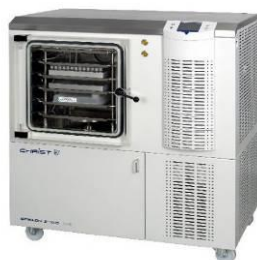
Figure 84: Freeze dryer used at ILVO
