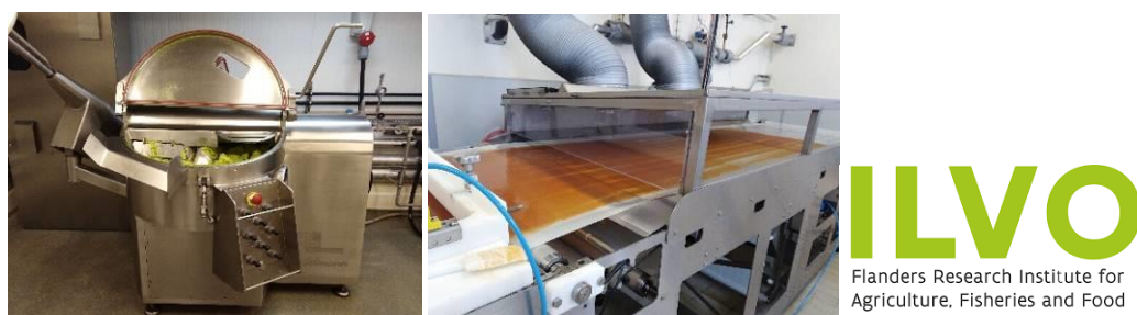
Figure 85: Vacuum-cooking cutter and Dry-On-Water used at ILVO
