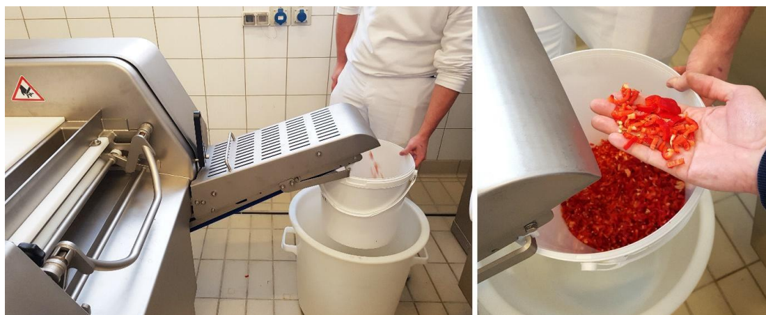
Fig. 1.20: The cube cutter dicer that was used for the experiments at ILVO Food Pilot.
