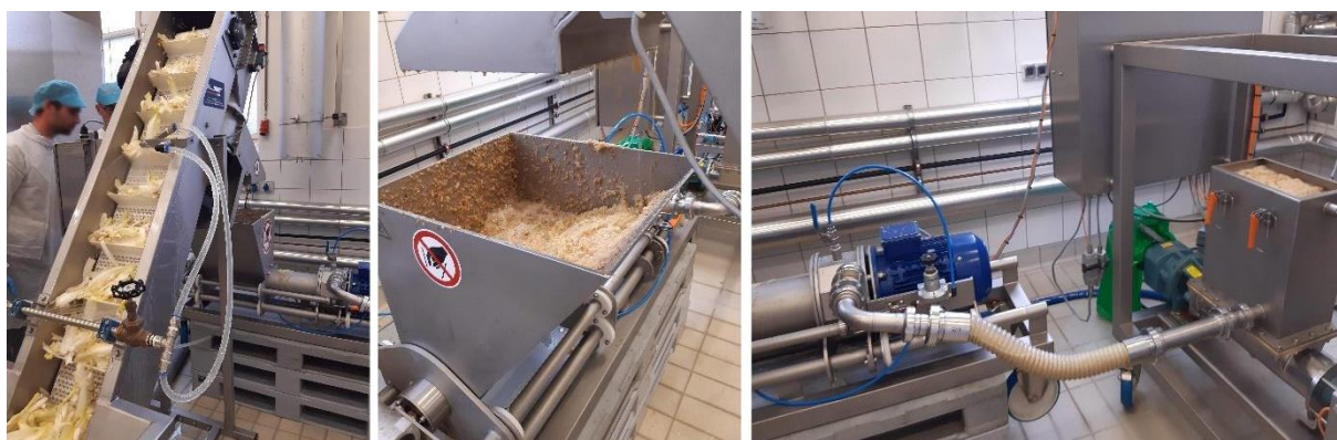
Fig. 2.16: Washed endive leaves are transported to the mixer (left), the mixer cuts the leaves to obtain a pulp (middle), the mixed leaves are pumped to the VaquillIQ® directly after mixing (right).
