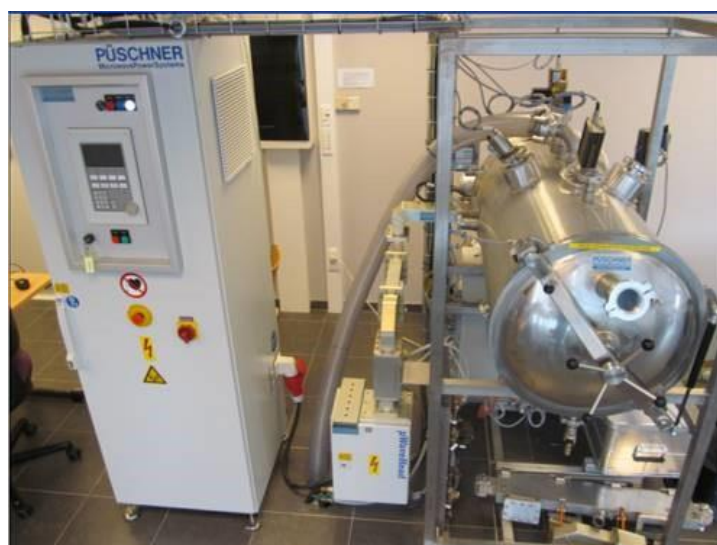
Fig.1.7: Microwave drying installation at VIVES. The same system was used for the Vacuum-microwave drying experiments
