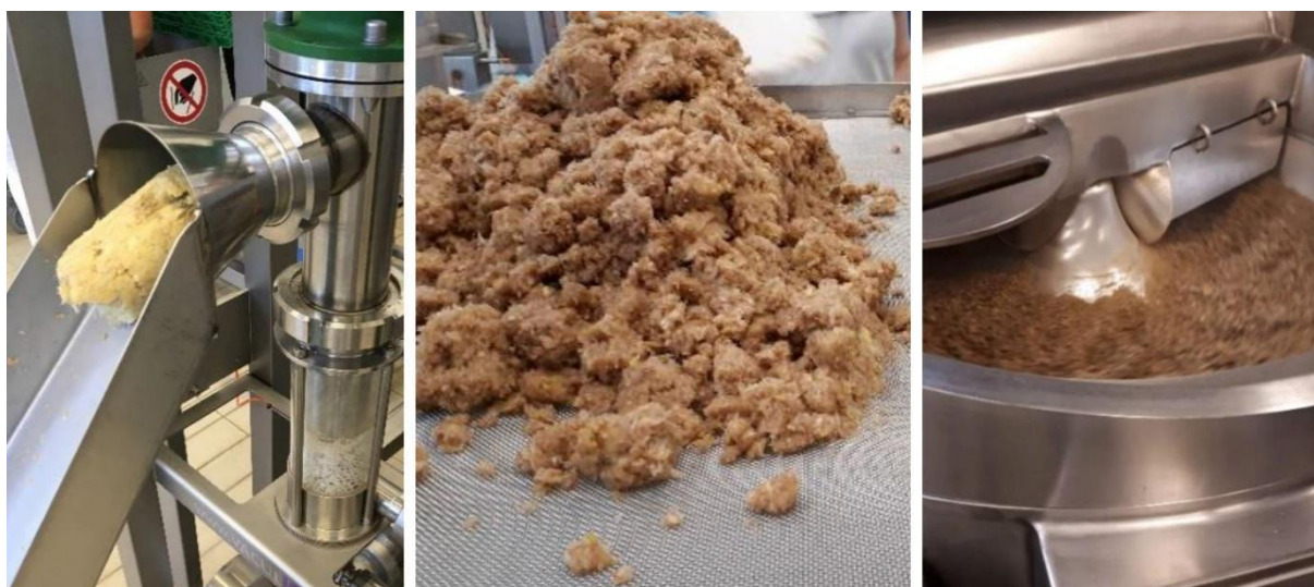
Fig. 2.18: Press cake coming out of the VaquiliQ® (left), dried press cake material (middle), and dried press-cake being cut to obtain fine material using a Seydelmann vacuum-cook-cutter.
