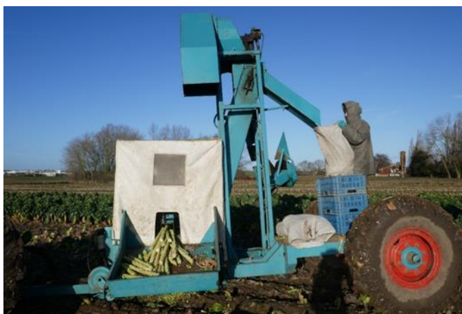
Figure 9 Adapted harvester in which sprouts are collected directly in the bag, while the stems are collected separately
