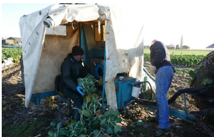
Figure 7 Harvesting machine for smaller cultivators separating stems, leaves and sprouts
