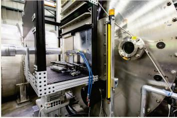
Sample area and detector tank of the Bio-SANS instrument at the High-Flux Isotope Reactor of Oak Ridge National Laboratory (Tennessee, USA).
