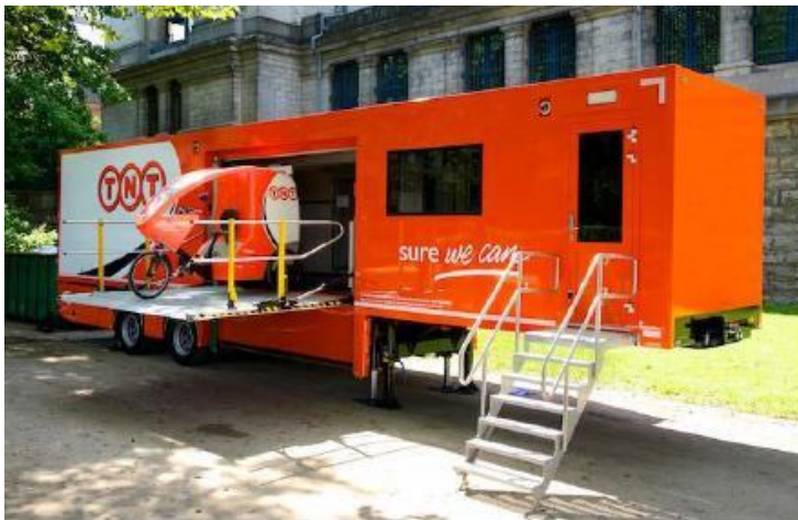
Figure 23: The Mobile Depot integrated with cargo bikes for last-mile delivery (TNT express and parcel pilot service)
