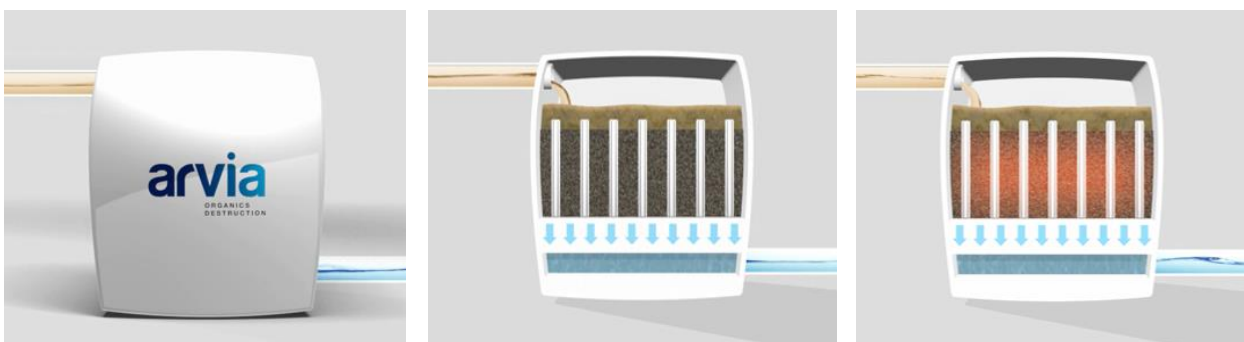
Figure 1. Modular design of Arvia's Nyex™ treatment system which treats water by adsorbing organic contaminants from the influent as it percolates the packed bed of Nyex™ particles, and the simultaneous passing of current ensures in situ oxidation of the adsorbed organic.
