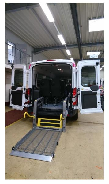
Fig. 2 – modification of car for PT use
