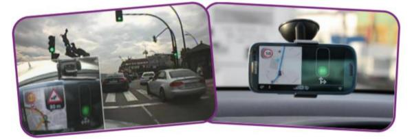
The pictures above show the HMI display combining in a map the RHW and EEIS services, with countdown of the time-to-green or time-to-red at equipped intersections in the city of Vigo.
