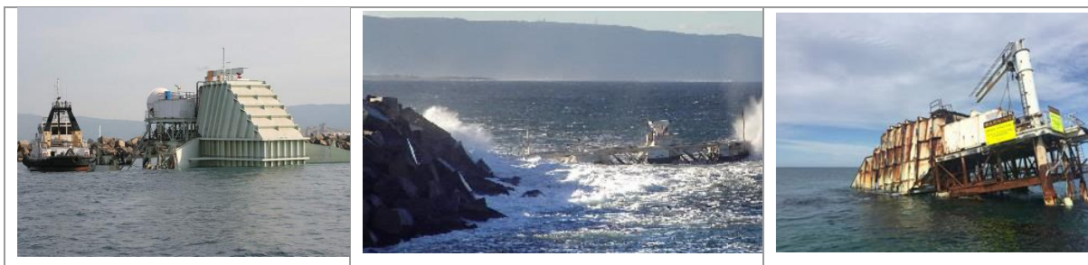
FIGURE 8 :AUSTRALIAN OCEANLINX (WAVE ENERGY - OSCILLATING WATER COLUMN), IN OPERATION, DURING THE MOORING LOSS IN 2010, 3 MONTHS AFTER DEPLOYMENT DURING A STORM & AS A STRANDED LIABILITY (HASHAM 2010, GRAYDIVINGSERVICES 2020)
