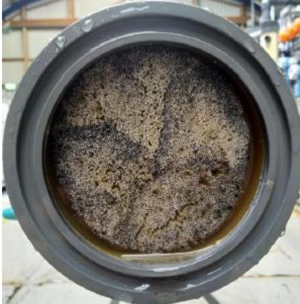
Figure 12 - Iron deposition on the NF membrane
