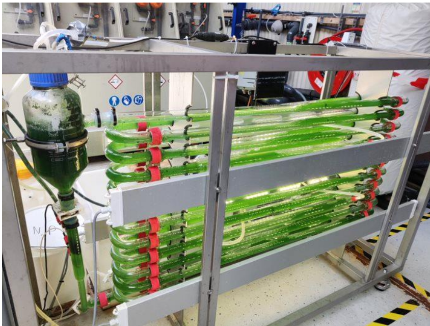
Figure 12 - Photobioreactor for algae cultivation
