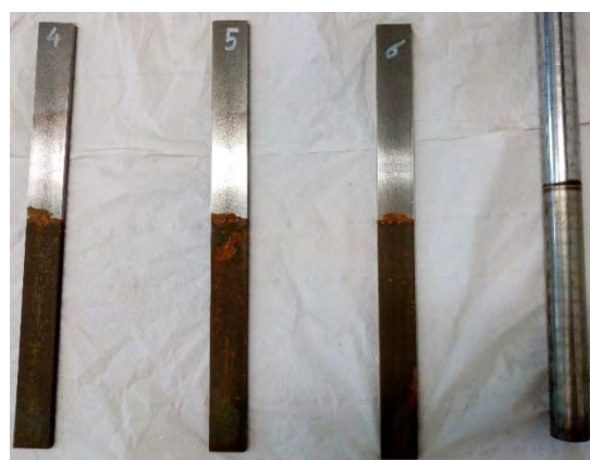
Figure 5 The degraded steel samples after TACM
