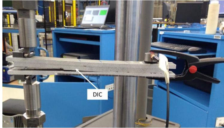
Figure 11 DCB testing setup
