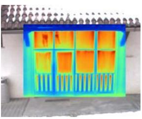
Figure 12: Thermal bridge on glass pane
