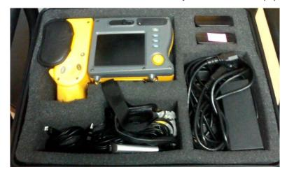
Figure 13: example of equipment (infrared camera) used for thermal inspection
