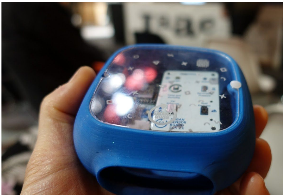
The Smart Citizen - Urban sensor board developed by FabLab Barcelona
