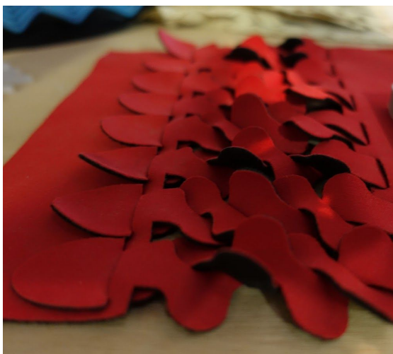
Other examples of innovation in textile design. Use of laser cutting (left) and 3D printing (right).
